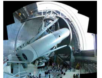
4.10 Palomar Observatory 200-inch Hale reflector, the world's largest telescope from 1948 to 1976. Courtesy of Palomar Observatory/California Institute of Technology
